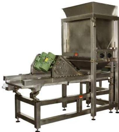
This model 510A breaks lumps of frozen goods. It consists of adjustable crushing rollers, a storage silo and a vibrating chute for the separation of small parts.
