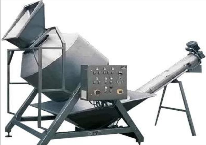
This model 500A creates a soft and intensive mixing of frozen foods. Due to the rotation of the mixing drum with the slanted welded plates, the product is optimally mixed without shear forces.
