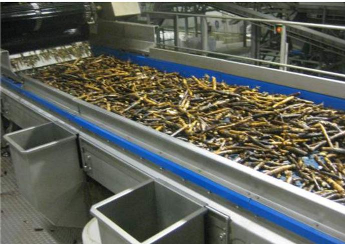
A sorting belt is a conveyor where workers can intercept lesser products and discard them in waste chutes. The conveyers are available in different lengths and widths depending on the task and customer needs.
