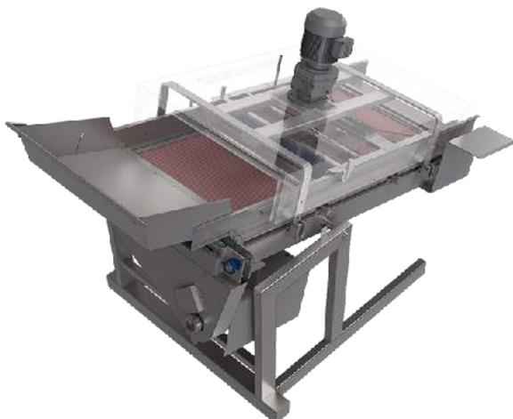
This machine (model 28BS / C) is used for the removal of the stems and washing of sweet and sour cherries, plums, olives, raisins, and also for the subsequent cleaning of beans pickles and onions. The capacity of fresh sour cherries with a full stem can amount to 1500 kg / h.
