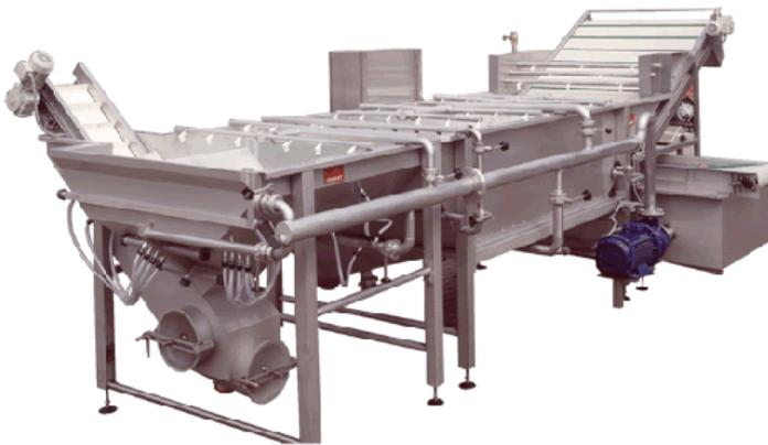
These machines are used for thoroughly washing beans, leafy vegetables and similar products. This machine has a length 6200mm and a width of 2590mm.
