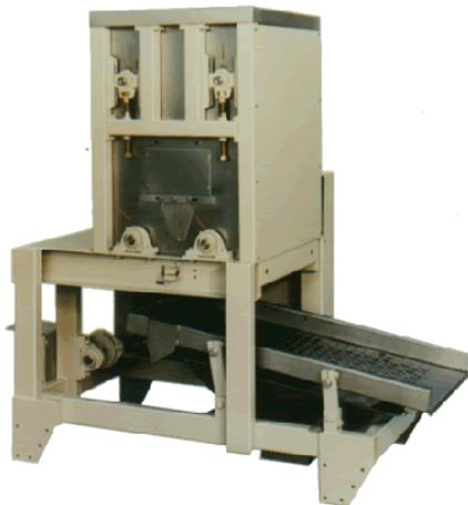
This machine (model 210H) is used for sharing and coring pointed peppers.
