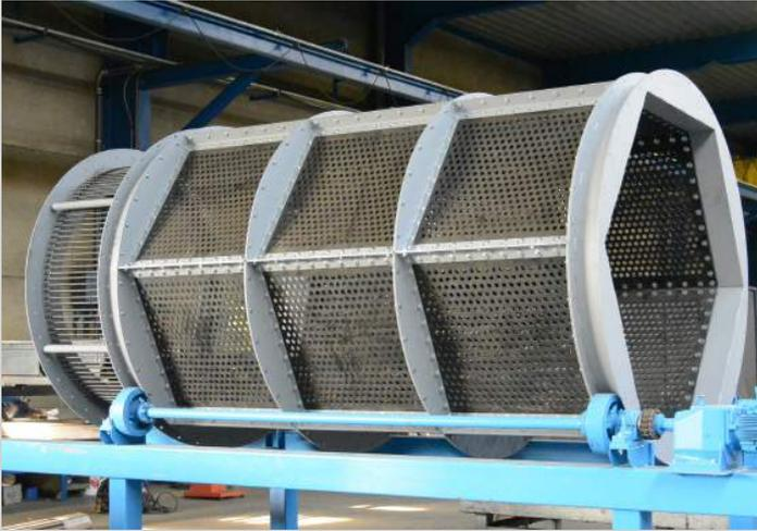
These machines screen small parts from plant products and are also suitable as remover of dry dirt.
