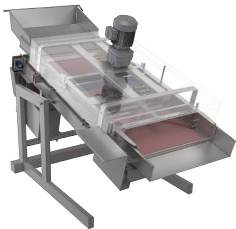
This machine (model 28BS / C) is used for the removal of the stems and washing of sweet and sour cherries, plums, olives, raisins, and also for the subsequent cleaning of beans pickles and onions. The capacity of fresh sour cherries with a full stem can amount to 1500 kg / h.
