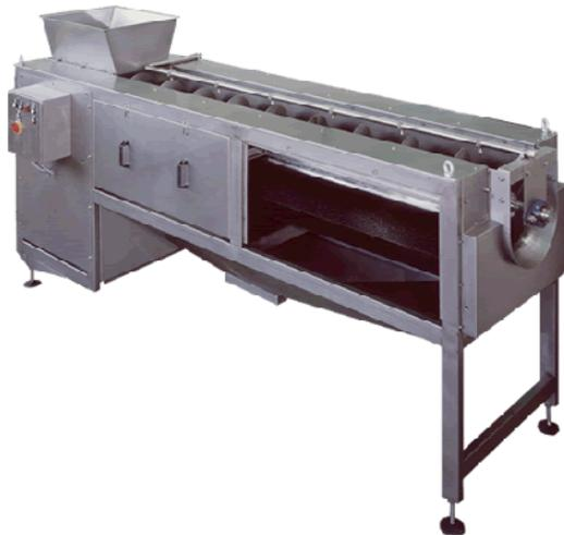
Machine (model 815) is used for washing and peeling fruit and washing vegetables, such as potatoes, carrots, turnips, beetroot, celery, after their peeling. Within the trough an adjustable screw is placed to regulate the capacity or throughput.
