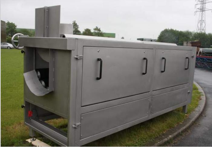
Machine (model 810) for washing and peeling horseradish. This machine has 8 peel brushes and has a capacity of 300kg.
