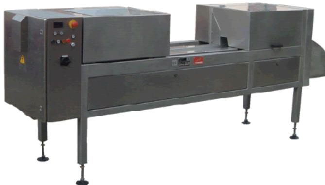
This design (model 26H) is characterized by its \_ perfectly smooth and accurate cut, and can therefore cut elongated products such as carrots, cucumbers, leeks, celery, rhubarb, beetroot (oblong varieties), headless asparagus, etc.
