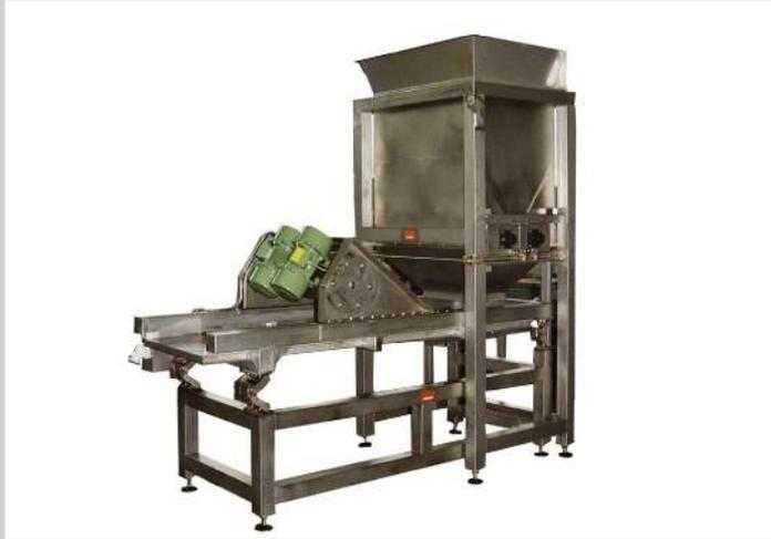
This model 510A breaks lumps of frozen goods. It consists of adjustable crushing rollers, a storage silo and a vibrating chute for the separation of small parts.
