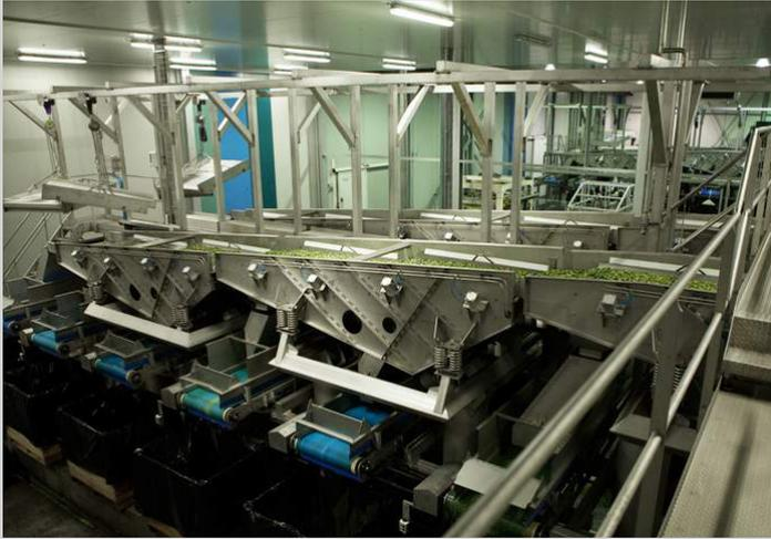
The model 207 transport system, distributes, sorts, dehydrates, etc.. using vibrations.
