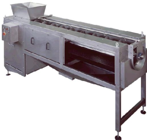
Machine (model 815) for washing and peeling fruit and washing after peeling vegetables like potatoes, carrots, turnips, beetroot, celery is used. Within the trough an adjustable screw is placed to regulate the capacity or throughput
