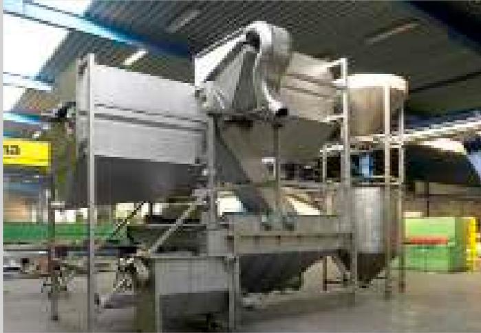
This machine with vertical screw separates stones and similar foreign materials through a simultaneous washing effect. The diameter can range from 1000mm to 3000mm.
