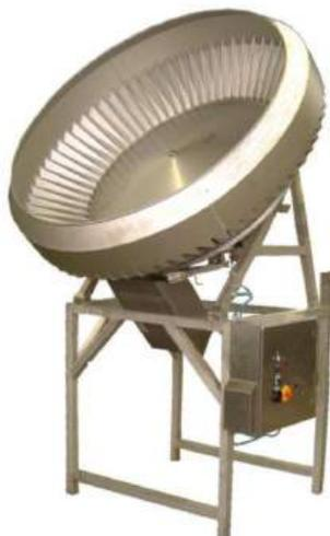
The machine 012A is suitable for cross cutting of whole green beans, wax beans and carrots with a diameter up to 20mm.
