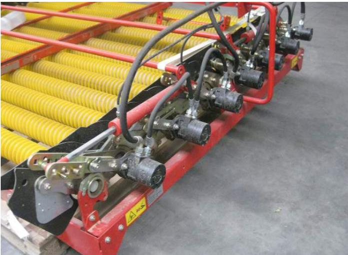
This machine is used to rid root vegetables of dirt using rollers. The product is gently but thoroughly cleaned.
