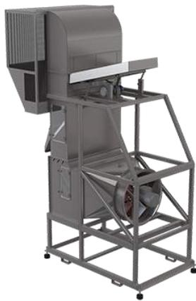
These machines (models 031C, 032A, and 033A) are suitable for dry cleaning of products, such as peas, green beans, white beans, lima beans, flageolet beans, etc. where lighter components are separated, by means of a fan, according to their density.
