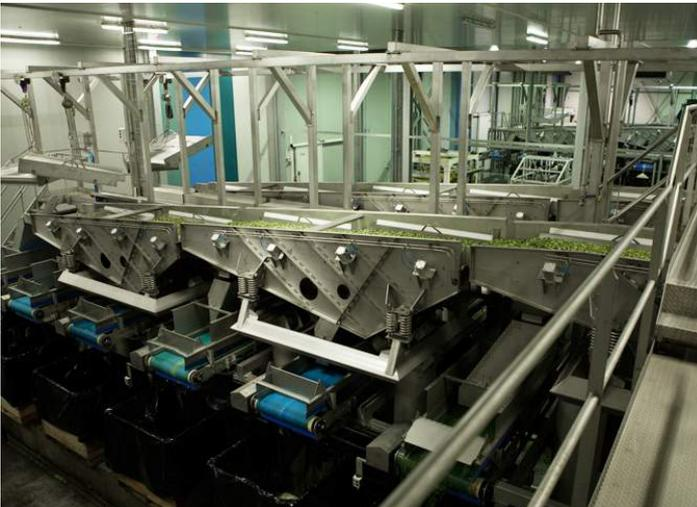
The model 207 transport system, distributes, sorts, dehydrates, etc, using vibrations.
