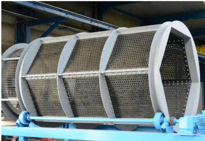
These machines screen small parts from plant products and are also suitable as removers of dry dirt.
