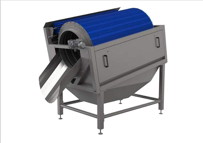
The machine 75B is ideal for debranching, destemming and topping beans.
