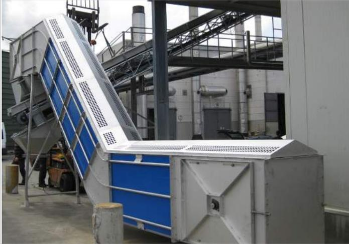
This redler allows transporting sticky products up without any dirt on the ground.
