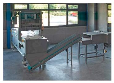
The machine is used to drill, the hearts of cabbages, and to separate and split the products.
