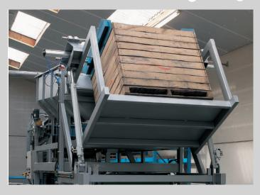
Crate turners are used to lift and empty crates, pallets and containers.
