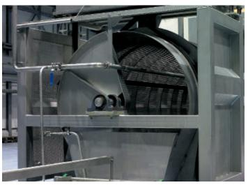
These machines (model 390) are ideal for pre-cleaning and washing of all root vegetables and tubers. For special applications, the drum can be divided into a wet and a dry area.
