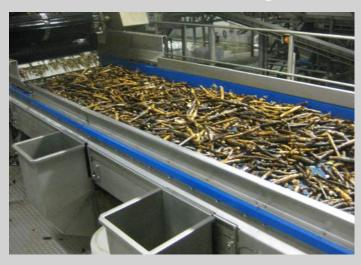
A sorting belt is a conveyer where workers can intercept lesser products and discard them in waste chutes. The conveyers are available in different lengths and widths depending on the task and customer needs.
