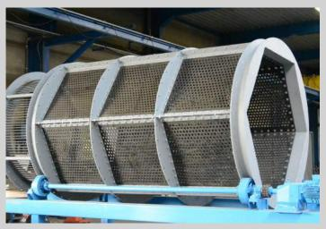
These machines screen small parts from plant products and are also suitable as remover of dry dirt. If necessary, the machine can be equipped with a stickdrum or a perforated drum.
