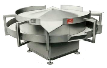
This model 213A is used for manual loading of up to four cauliflower splitters of type 211.
