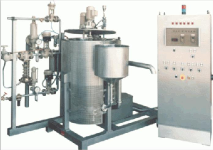
To complement our range of specialist products, the machine 159 CVT is available. This model is equipped with a double layered wall. The product can be alternately heated with steam or cooled with ice water.
