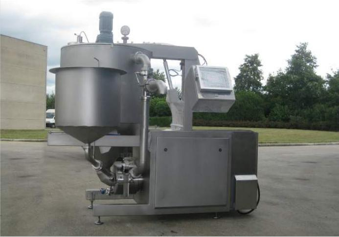
The mixer arrangement M is an additional component for all homogenizers. The mixing product is gently spread out and lumpy product components can be added and stirred. The use of an additional agitator may optionally be omitted. The machines are thus suitable for the mixing, stirring, homogenizing, and dispersing of liquid, viscous and highly viscous products.
