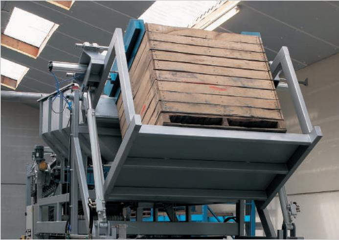
Crate turners are used to lift and empty crates, pallets and containers.
