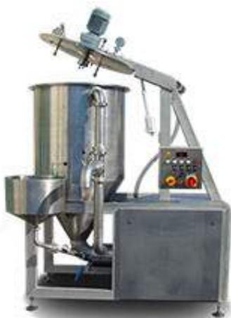
These machines are best suited for the production of homogeneous and dispersed products. This series has a vacuum device, homogenizing process is done in a vacuum. The product is continuously vented and therefore has a longer shelf life and is protected against oxidation and discoloration.
