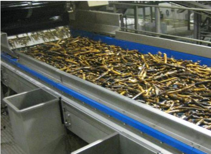
A sorting belt is a conveyor where workers can intercept lesser products and discard them in waste chutes. The conveyers are available in different lengths and widths depending on the task and customer needs.
