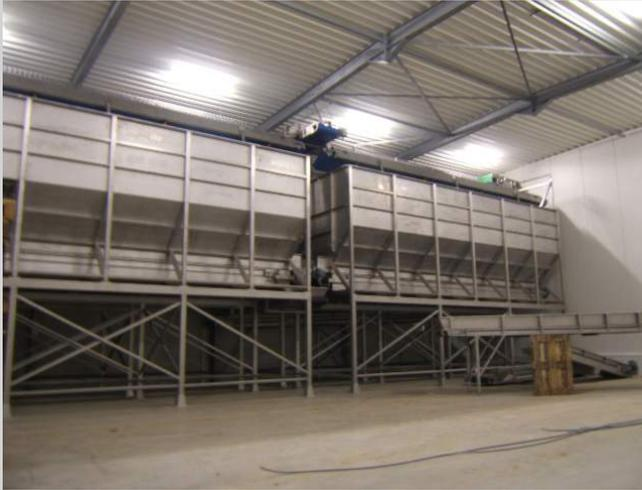
This construction precedes a processing line to provide a uniform and continuous flow of goods. Available in different shapes and sizes.
